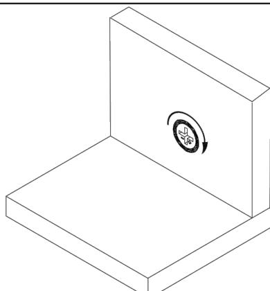
Use a Flat screwdriver to turn the Cam Lock clockwise one half turn so it locks onto the head of the Cam Pin. Turn only until it is snug. Over tightening could cause the Cam to bend or break. If it will not turn the full amount, turn the Cam Pin out (Counter-clockwise) one full turn, and try the Cam Lock again.
