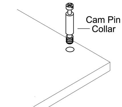
The Cam Pin is inserted into the flat side of a board, it is important that: The cam pin is kept vertical and is not put in on an angle. Cam pin is to be inserted up to collar Too far and it wont catch the Cam Lock (Do Not Overtighten) Not enough and the resulting product will not be stable.
